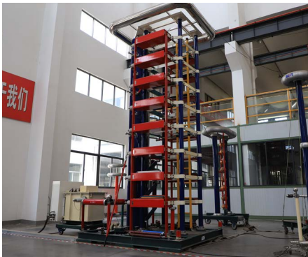
Impulse Test System
